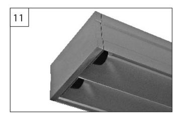
Push the end cap with stoppers into the top track and mark the location of the holes on the top track. Drill holes in top track and re-insert end cap with stoppers into top track and screw to blocking in ceiling with appropriate screws.
